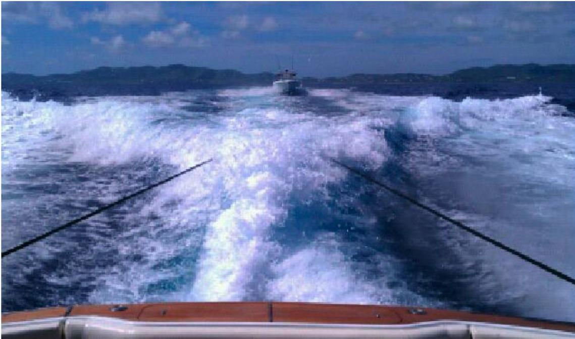
Above an example of a Fully Specified Ocean Tow Bridle, St. Croix USVI: 65 ft Hatteras Yacht towing a 32 ft Century. For this tow bridle the W.L. was chosen to be 10,000lbs minimum, which is the estimated fully loaded weight of the Century.
