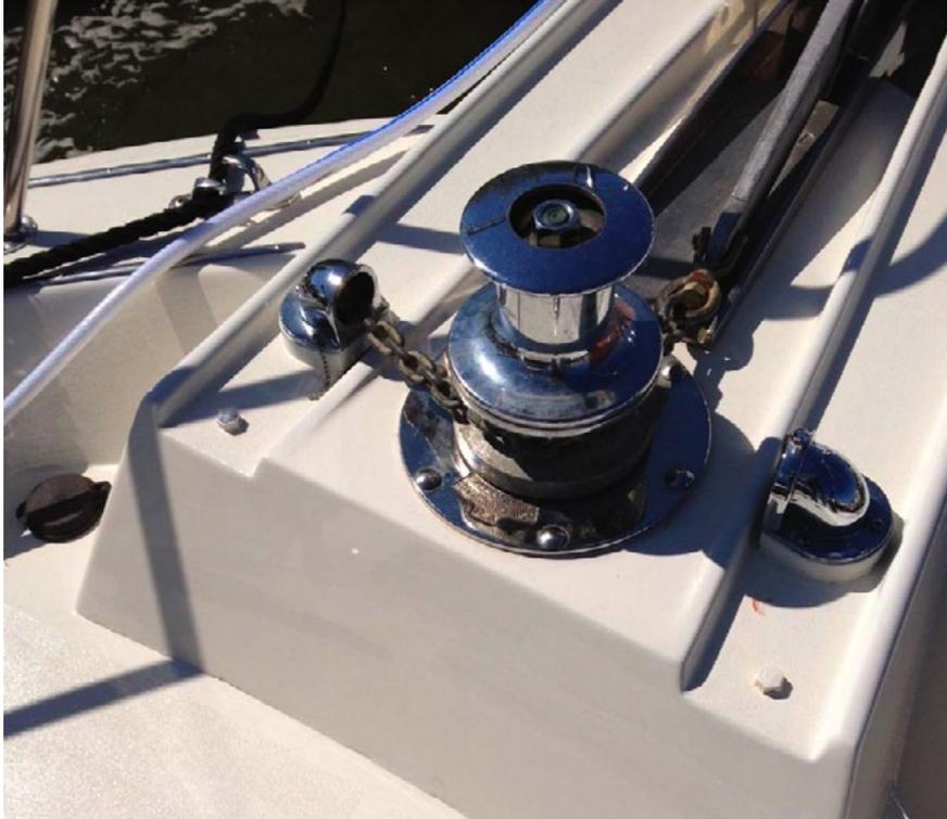
Above: An example of a Capstan on the bow area of a boat. The anchor rode drops down through the guide hole fitting into the anchor locker. In this example, a galvanized anchor shackle is connected to a standard type eye-and-jaw anchor swivel, which connects to the anchor.
