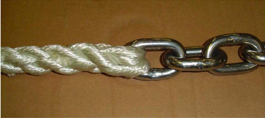
Above: A Direct Rope-to-Chain Splice most often applied to Windlass and Capstan applications utilizing 3-Strand Heat Set, 8-Strand Plait, or 12-Strand Plait white nylon rope. The chain link size is most often either BBB or G4HT. Consult the windlass or capstan manufacturer owner's manual to determine the rope and chain requirements.
