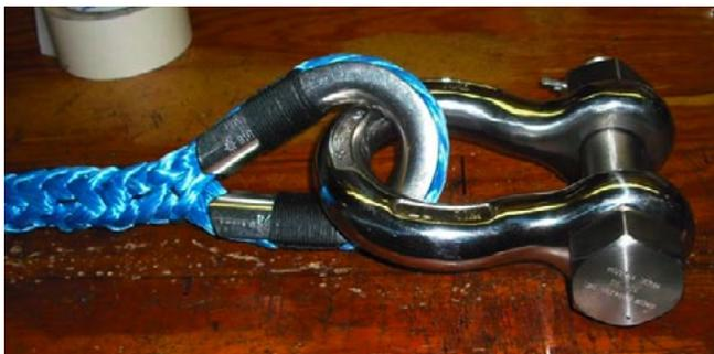
End view - 3/4" x 140 ft Tow Leg. This end provided with a heavy duty stainless steel thimble splice and a large 1-1/4" stainless steel bolted safety shackle for connection to the snubber shown below. Note the additional whipping used to keep the dyneema line seated in place. We specialize in stainless steel hardware for
