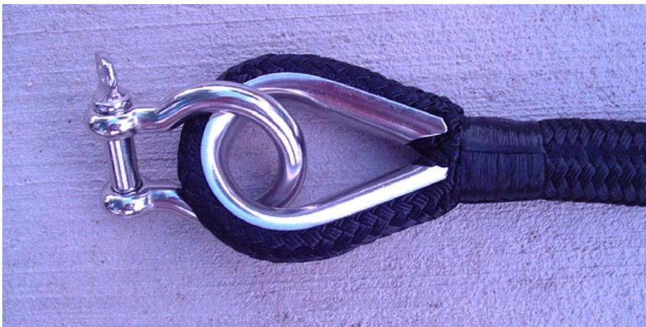
Above: A stainless steel thimble splice and bow shackle, which can be used to connect to a length of proof coil anchor chain or directly to an anchor. In this case the rope is black double braid nylon rope “yacht braid”. Note the hand sewing and whipping of the thimble splice. There are a wide selection of hardware and rope construction options available to pleasure marine applications (non-windlass and non-capstan applications). Give us a call to discuss your requirements.
