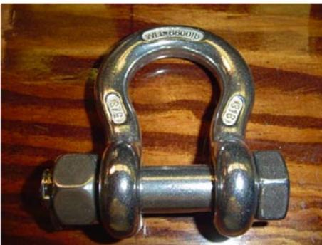
Year-long / permanent type moorings connections are often made using a Safety Bolted Shackle as shown here. This 5/8" stainless steel shackle has a bolted connection along with a cotter pin for extra security along with a higher working load than standard bow shackles.
