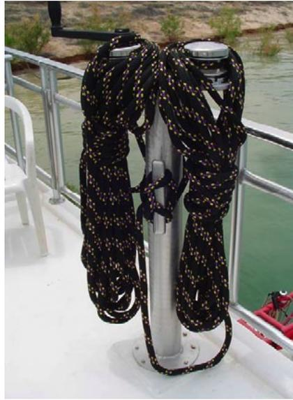
These two houseboats are outfitted with hand crank winches for taking the slack out of their anchor lines / shore lines. There are two aft winch stanchions, one on each side (port and starboard) of the houseboat for a total of four 3/4" custom colored double braid nylon anchor lines. The bitter end is on the boat through the winch, while a stainless steel thimble splice is on the shore for mechanical connection to the anchor / anchor rode chain using a stainless steel bow shackle. See below.
