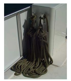
Above are two 3/4" x 200ft double braid nylon Shore Lines for the Bravada Houseboat below. The color combo is black/ gold snakeskin pattern.
