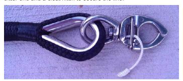
Above - Stainless steel thimble splice with a premium quality quick release snap shackle. Pull on the clasp to open the torsion bail. If your line is subject to twisting, then we recommend the use of a hook that is on a bearing. Make connections to your boat's bow eye using such a hook. Right - 1/2" & 5/8" lines with appropriately sized swivel eye hooks and anchor shackles.
