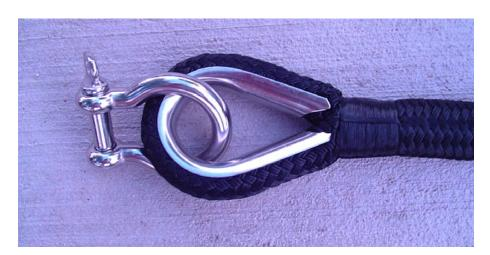
Above: A stainless steel thimble splice and bow shackle, which can be used to connect to a length of proof coil anchor chain or directly to an anchor. In this case the rope is black double braid nylon rope "yacht braid". Note the hand sewing and whipping of the thimble splice. There are a wide selection of hardware and rope construction options available to pleasure marine applications (non-windlass and non-capstan applications). Give us a call to discuss your requirements.
