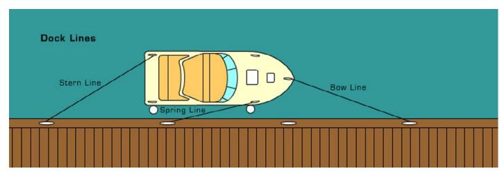
Typical Dock Lines Applied to starboard side of a boat.
