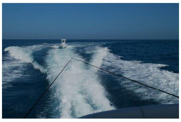
Above an example of a Fully Specified Ocean Tow Bridle: 58 ft Sovran Yacht by Tiara towing a 24 ft Center Console by Everglades The bridle's working load was chosen to be 4,500 lbs, which is the estimated fully loaded weight of the center console. Notice that the center console stays in the middle of the wake even as the Tiara is making a port side turn.
