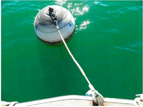
Above is an example of a houseboat mooring pendant. Denver Rope can custom assemble this type of pendant using stainless steel wire rope, heavy duty wire rope thimbles, swages, shackles, and or anchor swivels as the customer specifies. Consider that 12-Strand Dyneema Rope or Nylon Rope can be substituted for the wire rope shown.
