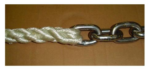
Above: A Direct Rope-to-Chain Splice most often applied to Windlass and Capstan applications utilizing 3-Strand Heat Set, 8-Strand Plait, or 12-Strand Plait white nylon rope. The chain link size is most often either BBB or G4HT. Consult the windlass or capstan manufacturer owner's manual to determine the rope and chain requirements.
