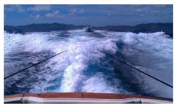
Above an example of a Fully Specified Ocean Tow Bridle, St. Croix USVI: 65 ft Hatteras Yacht towing a 32 ft Century. For this tow bridle the W.L. was chosen to be 10,000lbs minimum, which is the estimated fully loaded weight of the Century.
