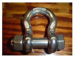
Year-long / permanent type moorings connections are often made using a Safety Bolted Shackle as shown here. This 5/8" stainless steel shackle has a bolted connection along with a cotter pin for extra security along with a higher working load than standard bow shackles.
