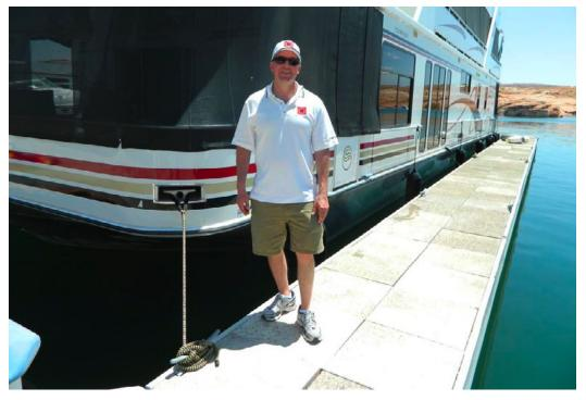
Above an example of a custom colored 3/4" X 15ft bow dock line with a 12" covered eye splice. A large houseboat like this one usually requires a minimum of four dock lines per side along with the required fenders / buoys and fender lines. If your lines are subject to chafing, then add chafe guard to protect the rope. This custom rope pattern is black/gold snakeskin.
