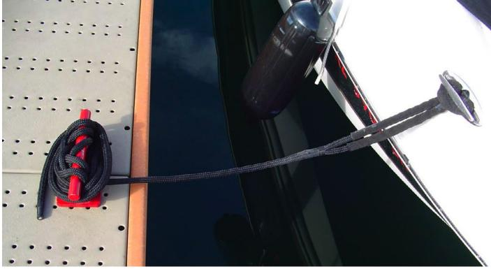
Above: A double braid nylon dock line for a boat in a slip. In this case, the boat's pop-out cleat fairlead hole is large enough for the covered eye splice to be pulled back through the center for a secure connection.
