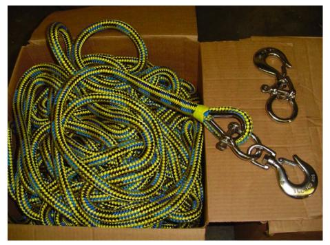
An example of a 3/4" x 150 ft custom colored double braid nylon anchor line or houseboat shore line. The 1/2" stainless steel bow shackle connects to a 3/8" stainless steel swivel eye hook, which connects to their anchor chain via another 1/2" stain steel bow shackle not depicted. Note that "Mooring Line" is a general term to include anchor lines, dock lines, shore lines, etc. Stainless Steel Hardware is standard on all our Mooring Lines.
